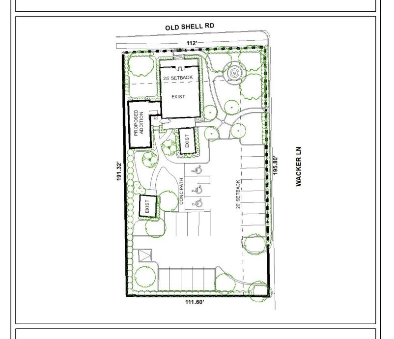
The site plan illustrates the existing structures, the proposed addition, proposed parking and setbacks.
