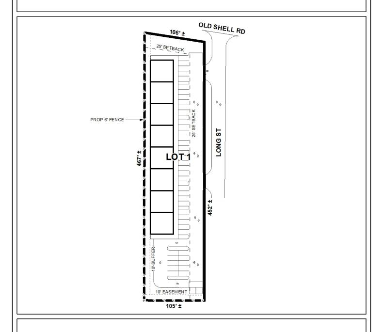
The site plan illustrates the proposed storage units, proposed parking, easement, buffer, and setbacks.
