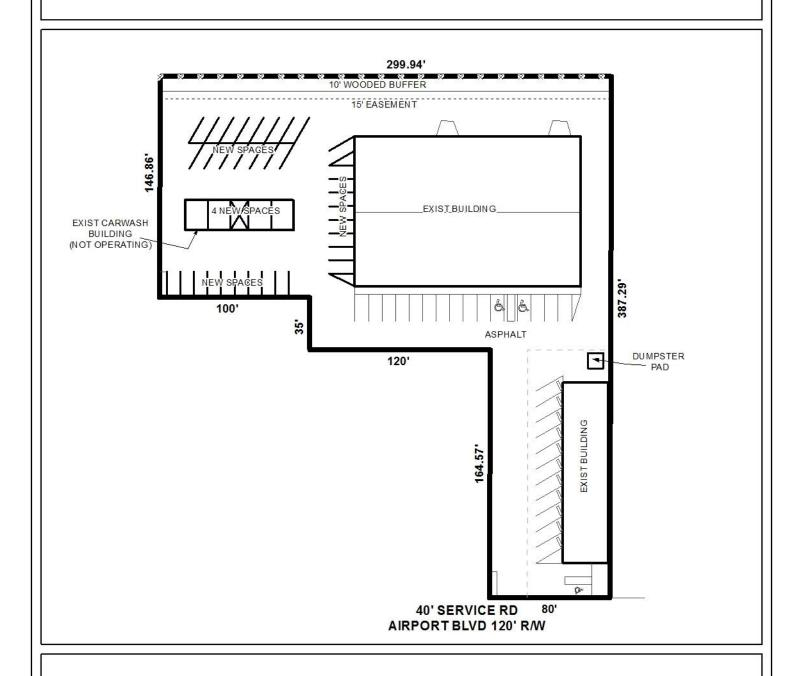
The site plan illustrates the existing buildings, new parking spaces, and easement.
