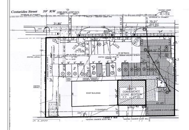
The site plan illustrates the existing building, parking, proposed addition, easements, and setback.
