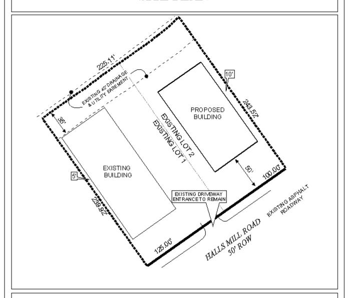
The site plan illustrates the old lot line, existing building, proposed building, drainage and utility easements, and driveway.
