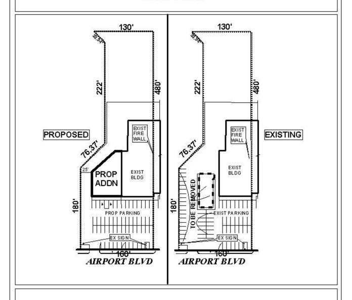
The site plan illustrates the existing buildings, parking, signs, and structures to be removed, along with the proposed parking and building addition.
