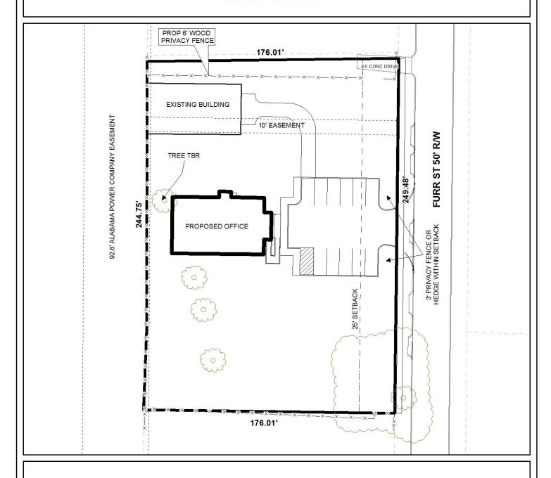
The site plan illustrates the existing building and drive, proposed building, parking, setback, and easements.
