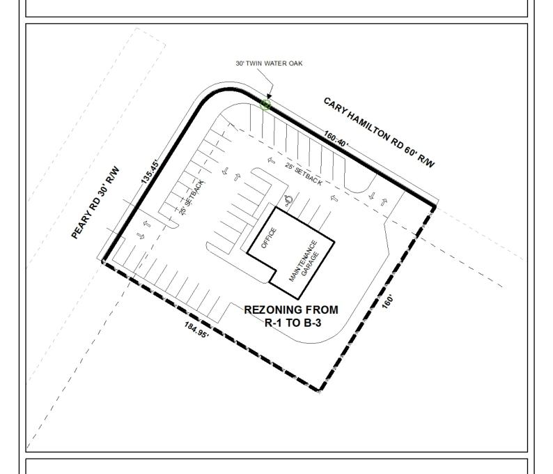
The site plan illustrates the existing structures, parking, setback, and area to be rezoned.
