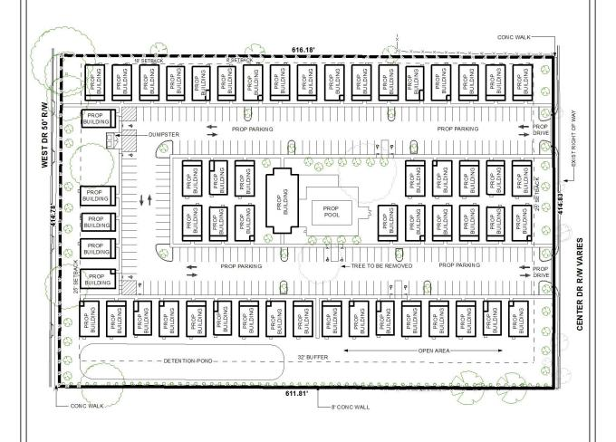
The site plan illustrates the proposed buildings, proposed parking, proposed drives, setbacks, buffer, and detention pond.
