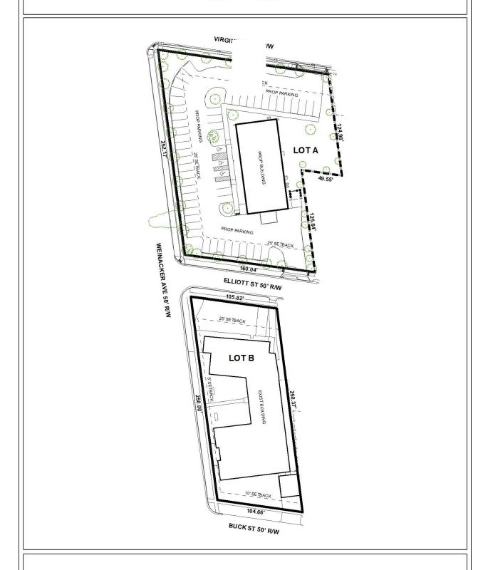
The site plan illustrates the existing building, proposed building, proposed parking, and setbacks.
