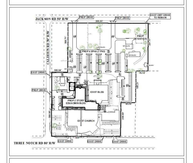
The site plan illustrates the existing improvements, proposed building, proposed parking areas, and proposed asphalt drives.
