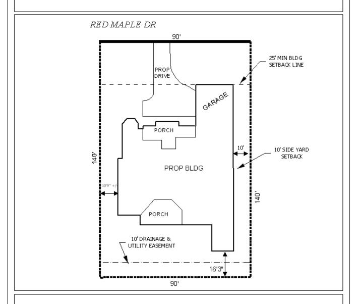
The site plan illustrates existing setbacks, easements, proposed building and drive.
