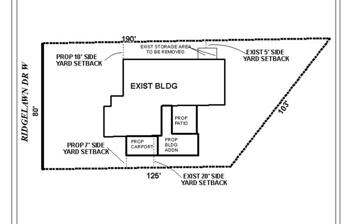
The site plan illustrates the existing buildings and setbacks along with the proposed additions, setbacks, and structures to be removed
