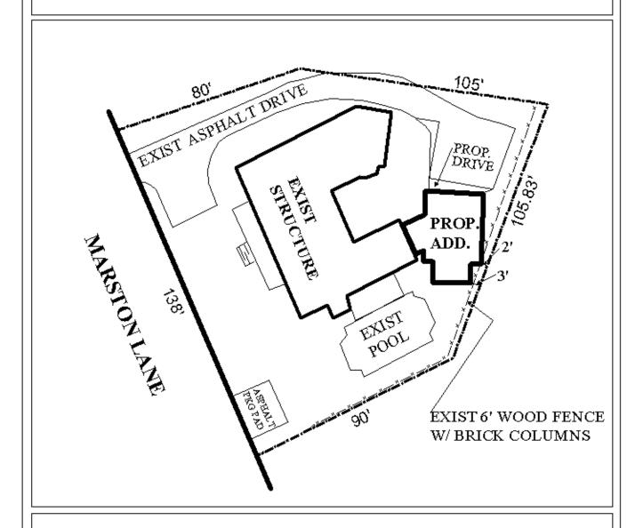
The site is located on the East side of Marston Lane, 155' North of Oakland Avenue. The plan illustrates the existing structure, drive, pool, and fence, along with the proposed addition and drive extension.
