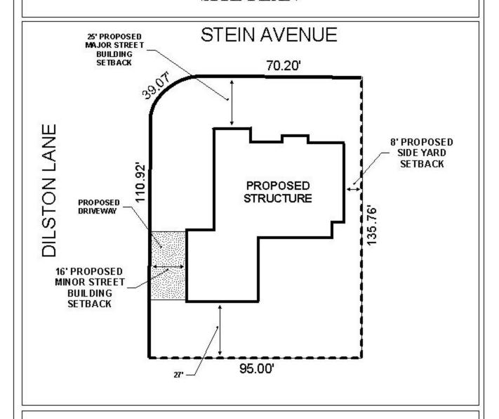
The site is located at the Southeast corner of Stein Avenue and Dilston Lane. The plan illustrates the proposed structure and setbacks.
