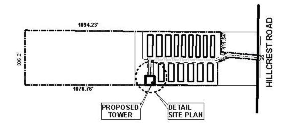
The site is located on the West side of Hillcrest Road, 950' North of Cottage Hill Road. The plan illustrates the existing structures, along with the proposed tower.
