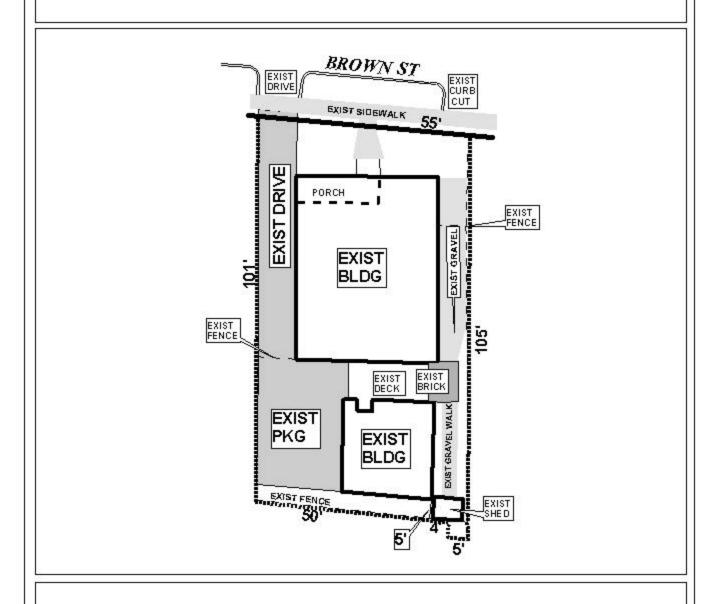
South side of Brown Street, 50' East of S Lafayette St, the site plan illustrates the existing buildings, drives, fencing, and gravel along with the proposed rear yard setbacks.
