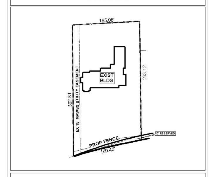
North side of Old Shell Road, 210' West of Ridgelawn Drive West, the site plan illustrates the existing building, easements, and proposed fence location
