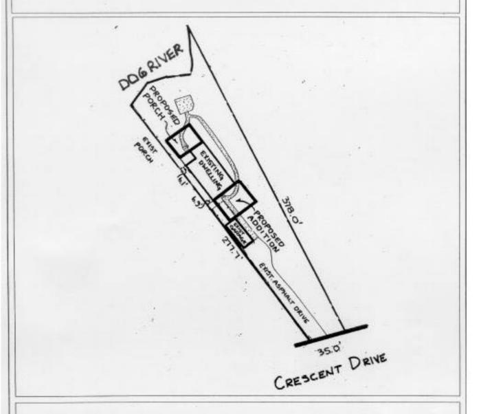
The site is located on the North side of Crescent Drive North, 60' East of Crescent Drive West. The plan illustrates the existing structures and drive, along with the proposed addition and porch.
