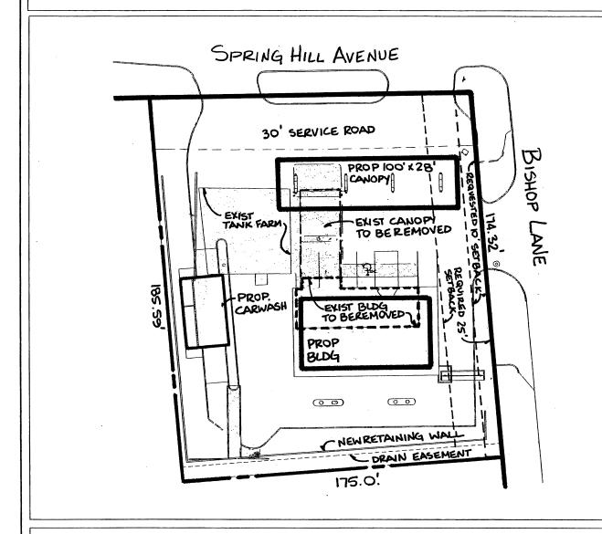
The site is located on the Southwest corner of Spring Hill Avenue and North Bishops Lane. The plan illustrates the existing structure and canopy, to be removed, and existing tank farm. Also shown on the plan are the proposed structure and canopy.
