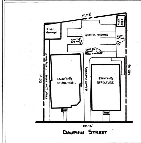
The site is located on the North side of Dauphin Street, 198' West of North Bayou Street. The plan illustrates the existing structures along with the proposed gravel parking and drive.
