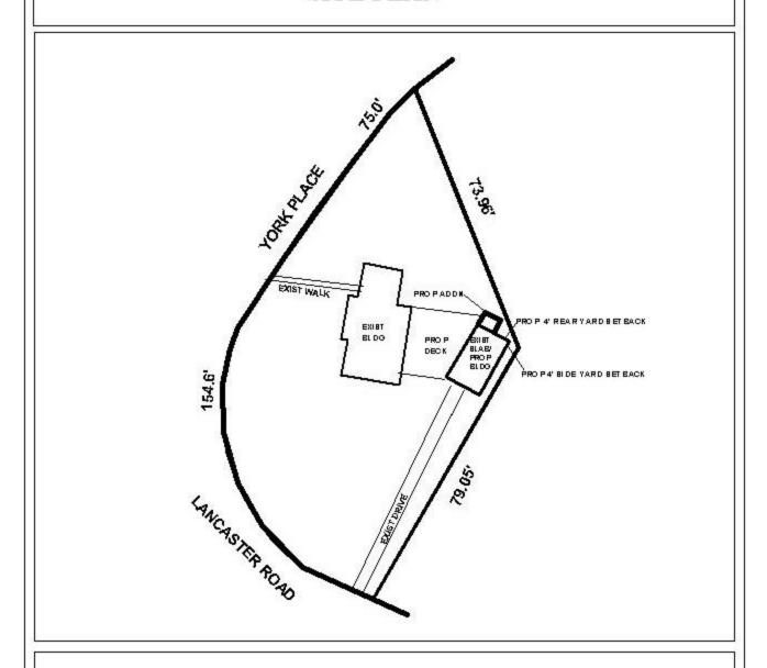
Southeast corner of Lancaster Road and York Place. The site plan illustrates the existing building and slab, proposed carport, deck, and carport addition.
