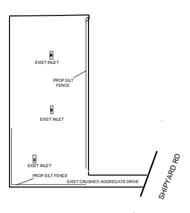
Westside of Shipyard Road, 1115' North of Higgins Road. The site plan illustrates the existing crushed aggregrate drive, existing inlets, and proposed silt fences.
