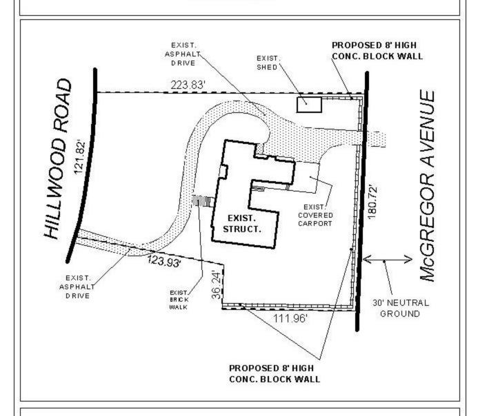
The site is located on the East side of Hillwood Road, 175' South of Vickers Place, extending to McGregor Avenue. The plan illustrates the existing and proposed structures.
