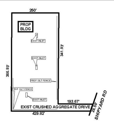
West Side of Shipyard Road, 1115' North of Higgins Road, the site plan illustrates the existing crushed aggregate drive, proposed fencing and existing inlets.
