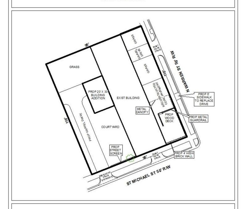
The site plan illustrates the existing building, proposed addition, and proposed drive.
