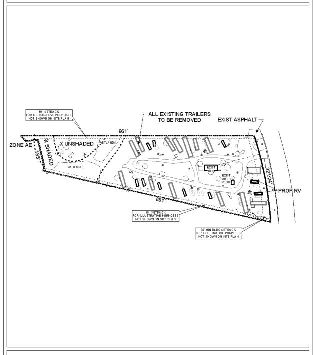
The site plan illustrates the existing development, proposed trailers to be removed, and proposed rv sites.
