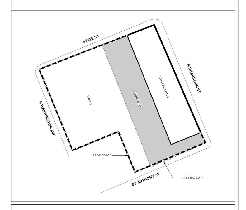
The site plan illustrates the existing building, drive, and proposed fencing and gate.
