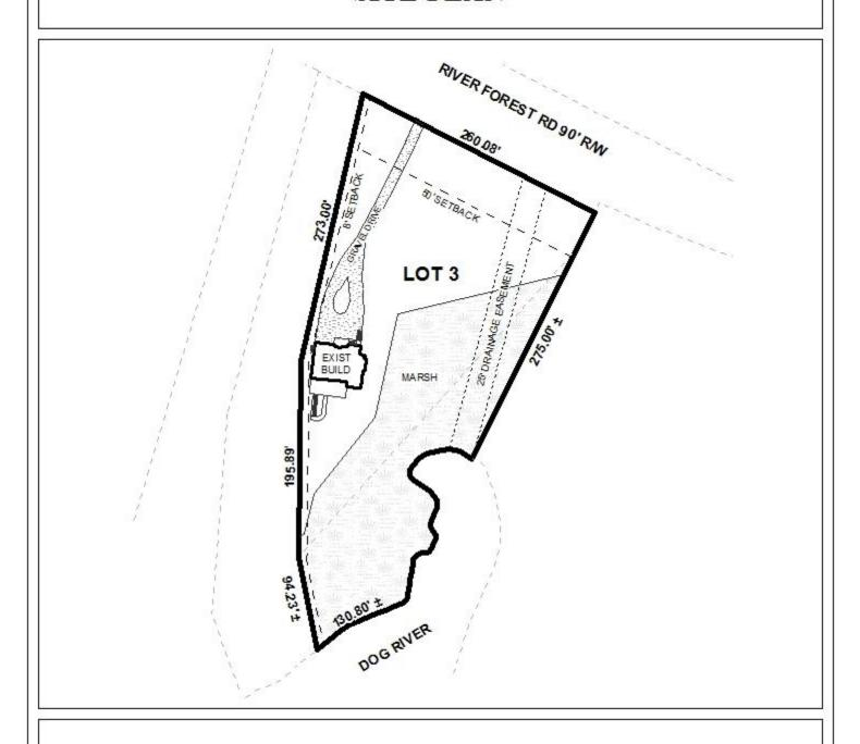
The site plan illustrates the existing building, gravel drive, setbacks, and easements.
