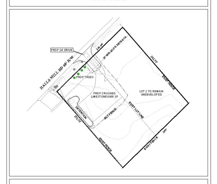
The site plan illustrates the proposed storage yard with aggregate surface.
