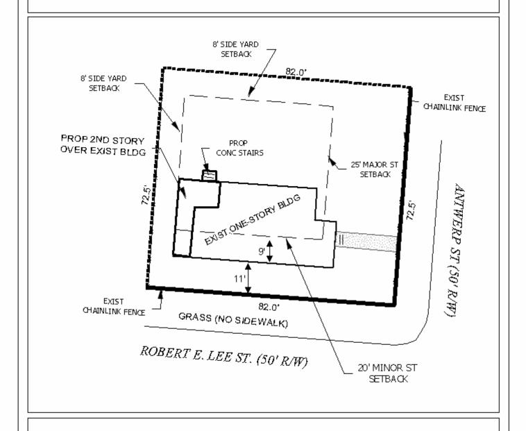
The site plan illustrates the existing building, proposed addition, and building setbacks.
