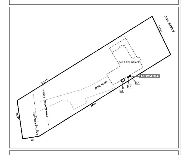
The site plan illustrates the recently constructed residence and condenser units.
