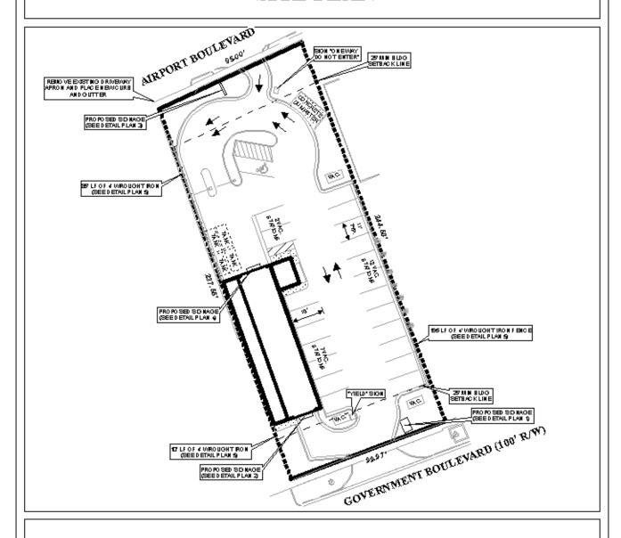
This site plan illustrates the proposed signs, fence, and car wash configuration. See detail site plans for sign designs.
