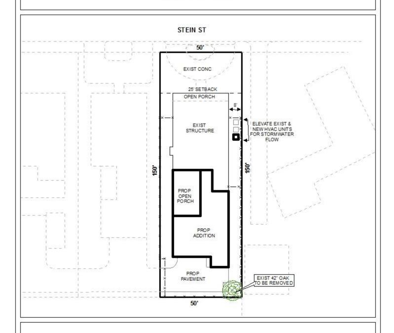
The site plan illustrates the existing building, proposed additions, setback, exist AC units, and a new AC unit.
