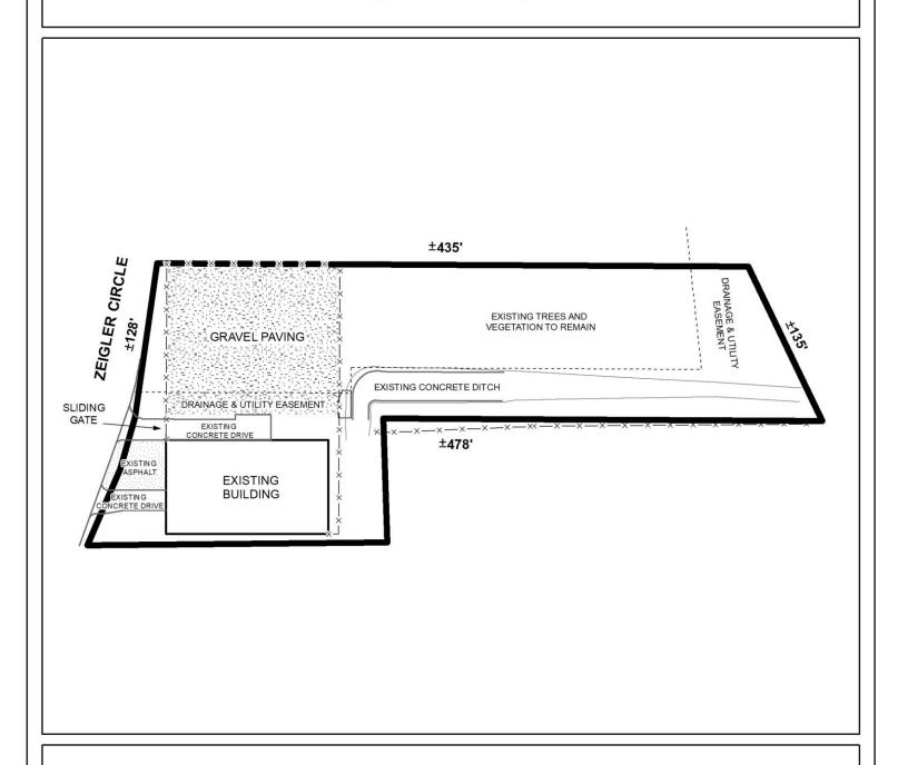
The site plan illustrates proposed gravel paving and existing building, vegetaion and easement.
