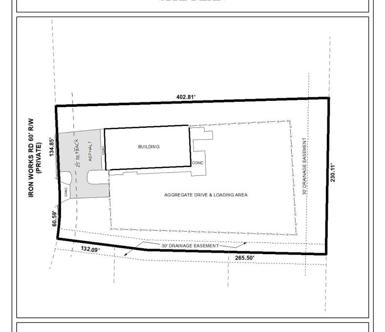
The site plan illustrates the existing building, loading area, setback, and easements.
