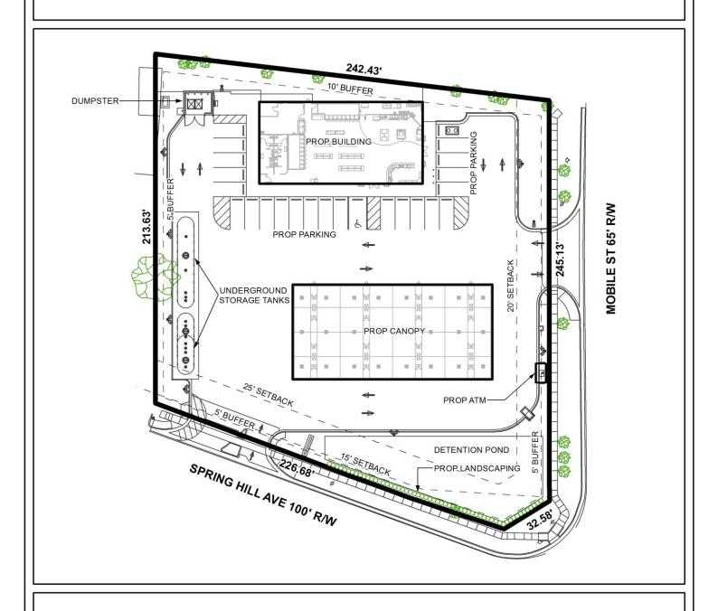
The site plan illustrates the proposed building, proposed canopy, proposed parking, proposed detention pond, setbacks, proposed landscaping, and proposed atm machine.
