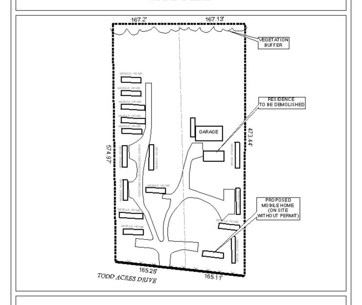
The site plan shows existing and proposed mobile homes, drive, and building to be demolished.
