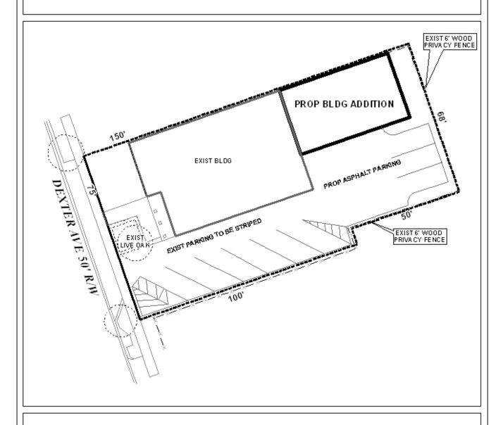
The site plan illustrates the existing development, proposed building addition, and proposed parking.
