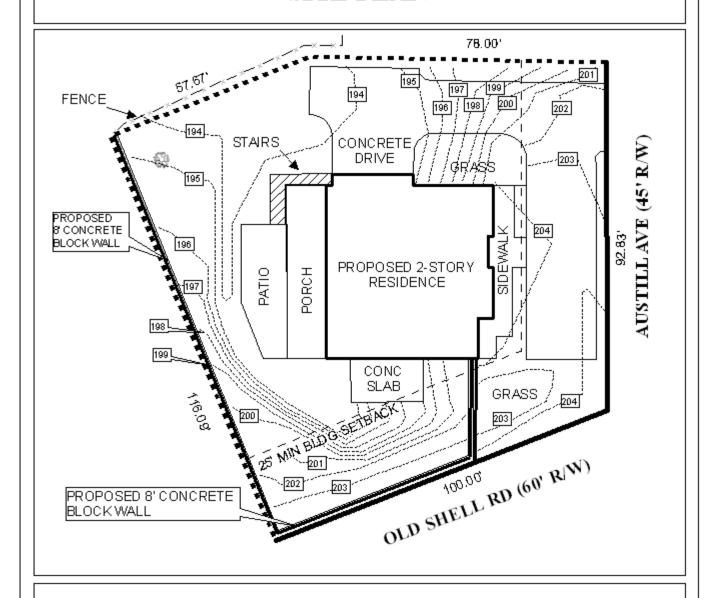
This site plan illustrates proposed structures and surrounding elevation (feet).
