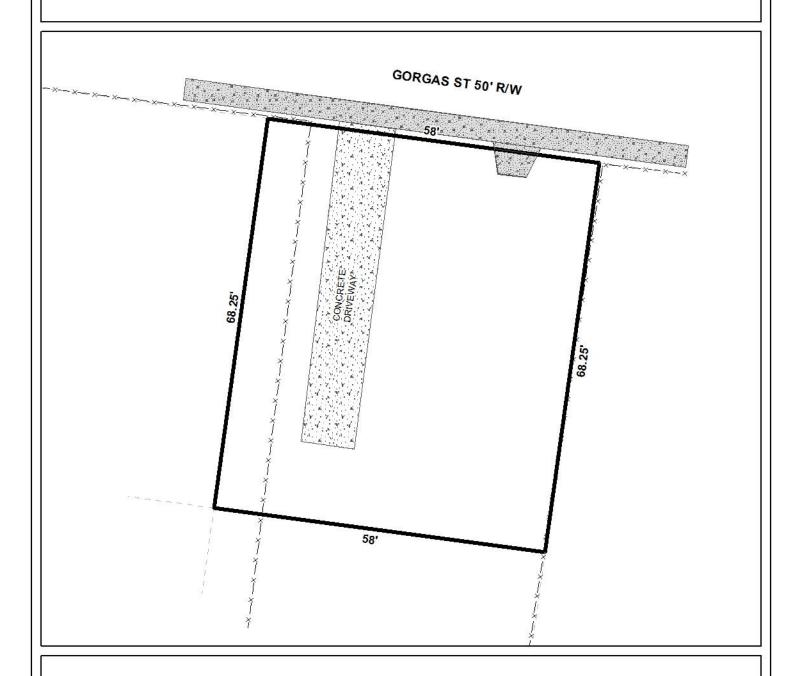
The site plan illustrates the concrete driveway and fences.
