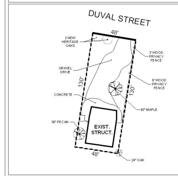
The site is located on the South side of Duval Street, 100' East of Amsterdam Court. The plan illustrates the existing structure and parking.
