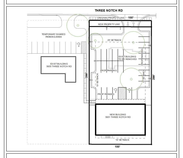
The site plan illustrates the exsiting building to be removed, new building, proposed parking, and the temporary shared parking area.
