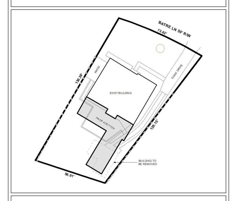
The site plan illustrates the existing building, existing drive, building to be removed, and proposed addition.
