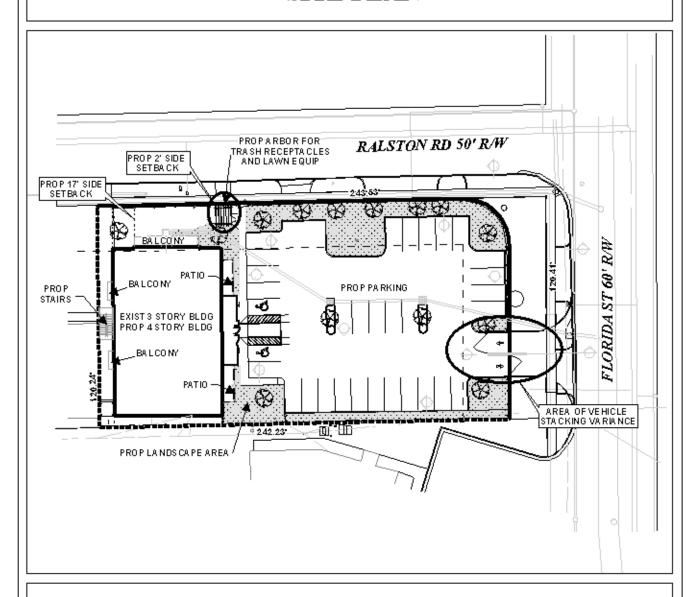
The site plan illustrates the existing building with proposed story addition, stairs, balconies, and patios. A proposed arbor and proposed parking are also illustrated on the plan.
