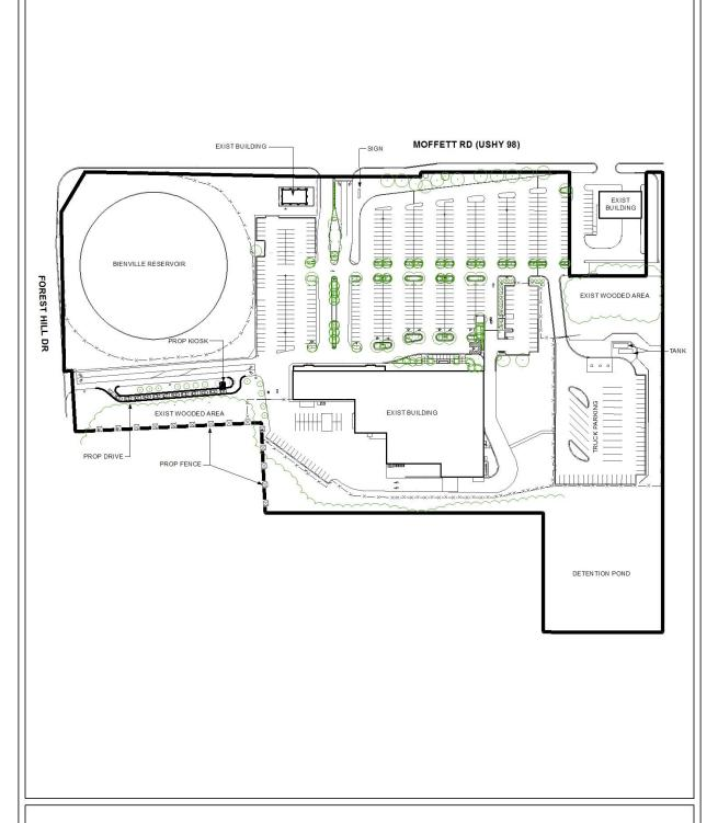
The site plan illustrates the existing buildings, existing wooded areas, existing parking, proposed drive, proposed kiosk, and proposed fences.
