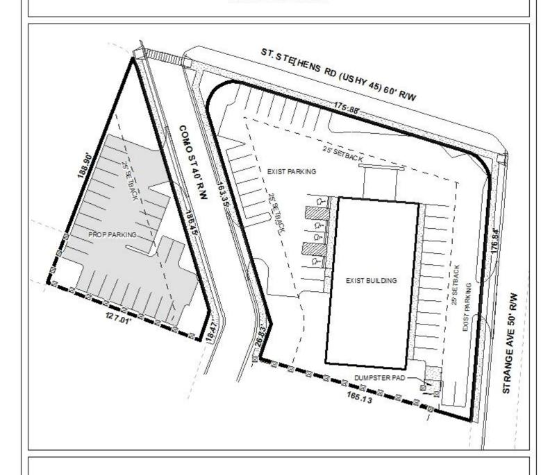
The site plan illustrates the existing building, existing parking facility, and proposed off-site parking facility.
