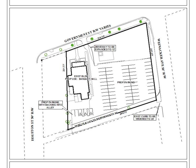
The site plan illustrates the existing building, proposed parking, and existing alley to be widened.
