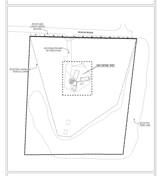
This site plan illustrates the existing lot configuration and proposed landscaping buffer. See detail site plan and tower detail.
