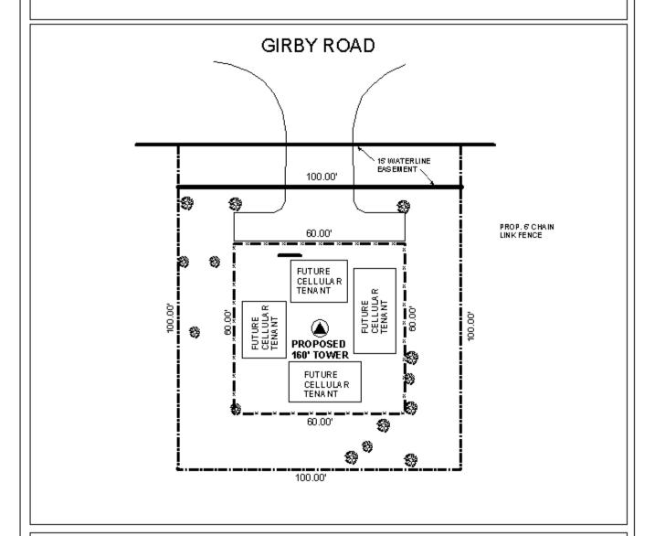
The site is located on the South side of Girby Road, 1/2 mile East of Hillcrest Road. The plan illustrates the proposed tower and easement.
